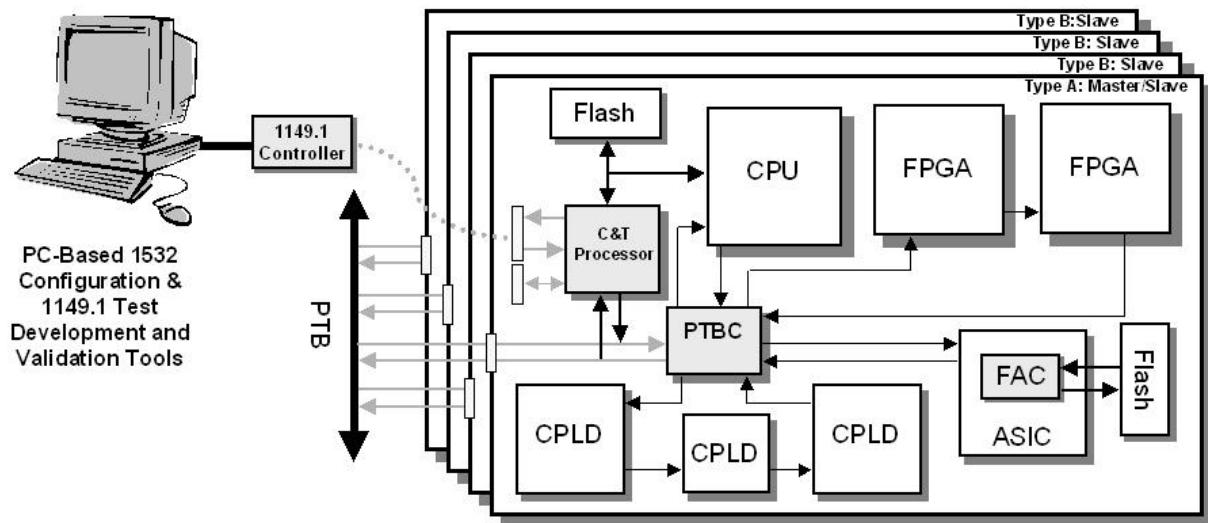
**Figure 7.** Top-Level Block Diagram of the C&T Processor
